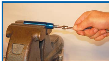
STEP 2 Flare braid using a twisting motion.
