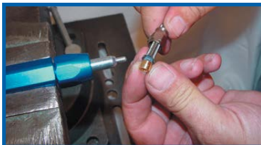
STEP 3 Insert olive on tube and under braid.
